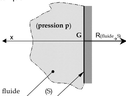
$$\{T_{\text{fluide} \rightarrow S}\}_G = \left\{ \begin{array}{l} \vec{R}(\text{f} \rightarrow S) = -p \cdot S \cdot \vec{x} \\ \vec{M}_G(\text{f} \rightarrow S) = \vec{0} \end{array} \right\}_R$$
