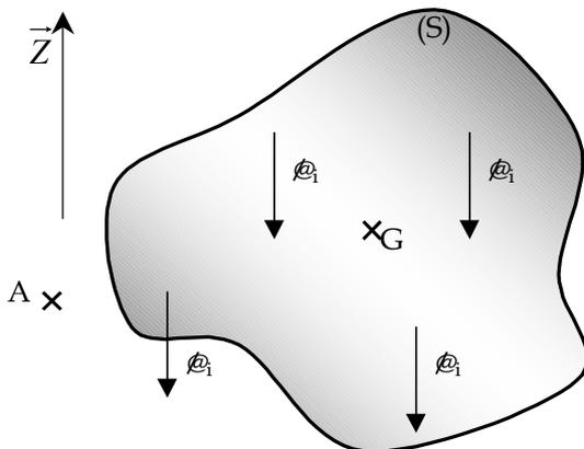
$$\{\mathcal{T}_{\text{pesanteur} \rightarrow S}\} = \left\{ \begin{array}{l} \vec{R}_{(\text{pes} \rightarrow S)} = \sum_{i=1}^n \vec{p}_i = \vec{P} \\ \vec{M}_G(\text{pes} \rightarrow S) = \sum_{i=1}^n (\vec{AM}_i \times \vec{p}_i) \end{array} \right\}_R$$
